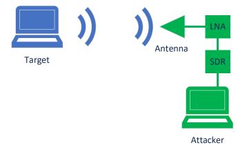
Figure 1: Radio setup
