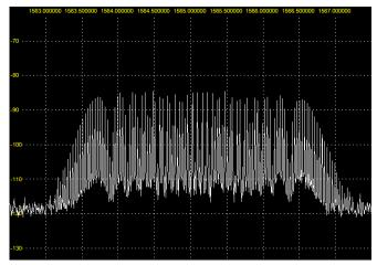
*Figure 7: Received clock signal 50 feet away from the desktop computer. Frequency span between 1562.5 MHz and 1567.5 MHz.*
