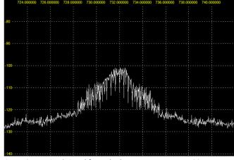
Figure 9: Received signal from the laptop computer at 732MHz (Transmission clock set to 1465.25). Frequency span between 722 MHz and 742 MHz.
