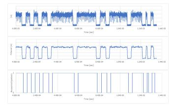
Figure 8: A sample for received and processed symbols. The upper graph shows sample of the absolute value of the received vector. The middle graph shows the data after filtering. The lower graph shows the symbols recovered from the data.
