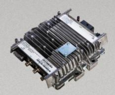
The Modular Telematics Gateway integrates GNSS, mobile connectivity and on-board machine communications via CAN, Ethernet, and RS-232. It's ideally suited for advanced telematics applications such as machine health monitoring, advanced logistics, and remote diagnostics.
